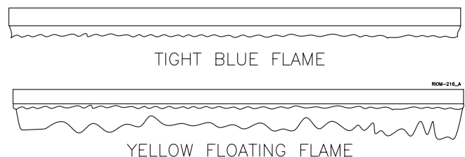
Figure 26 - Main Burner Flame
